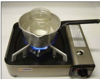
Figure 1. Flash-heat experiment using simple equipment
